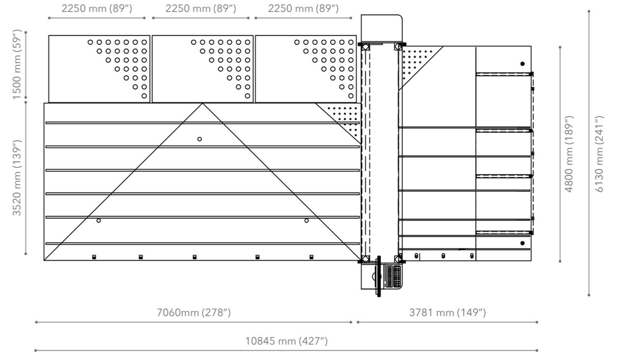
Machine overall dimension valid also for Dual Line with BCS/EVO • Ingombro macchina valido anche per Dual Line con BCS/EVO
