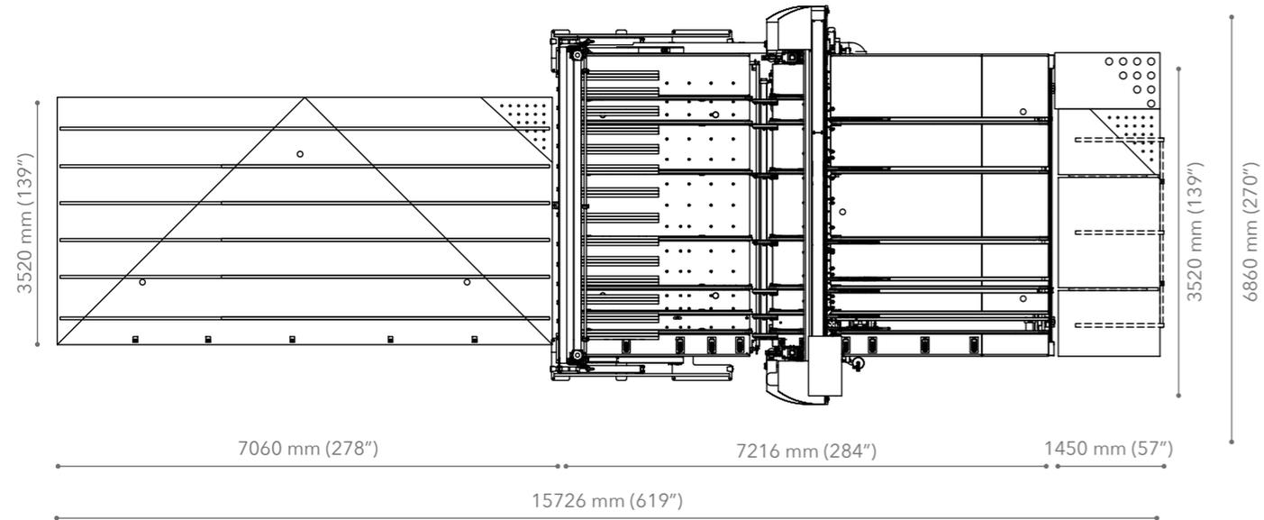
Machine overall dimension valid also for Dual Line with BCS/EVO • *Ingombro macchina valido anche per Dual Line con BCS/EVO*
