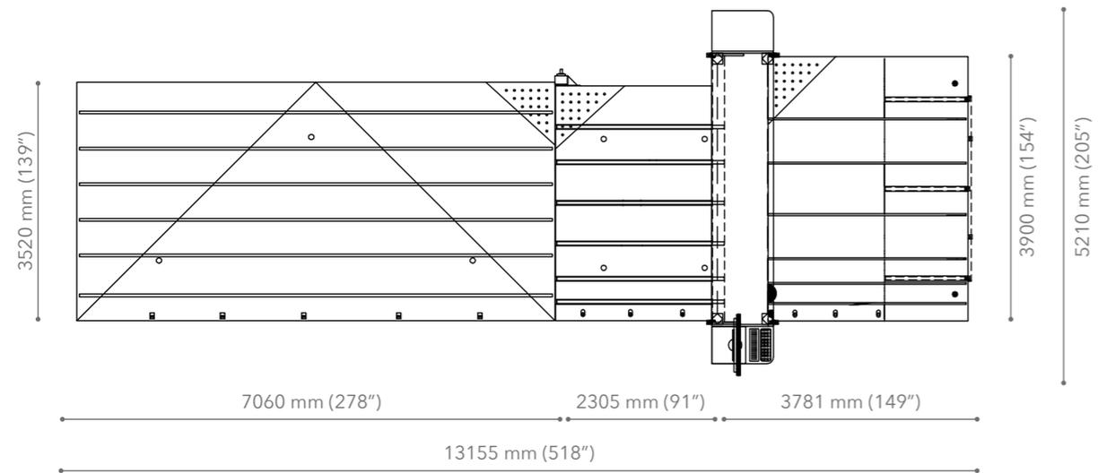
Machine overall dimension valid also for Dual Line with BCS/EVO • Ingombro macchina valido anche per Dual Line con BCS/EVO
