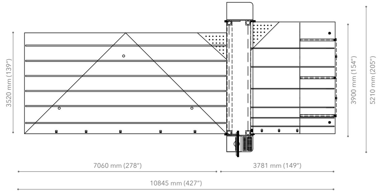
Machine overall dimension valid also for Dual Line with BCS/EVO • Ingombro macchina valido anche per Dual Line con BCS/EVO
