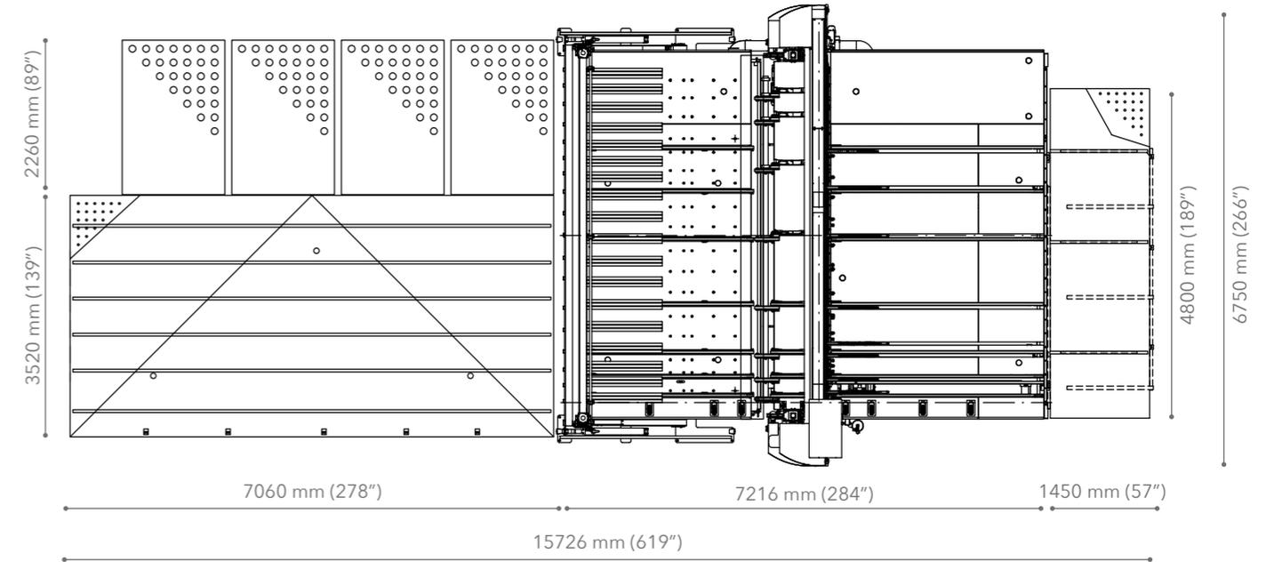
Machine overall dimension valid also for Dual Line with BCS/EVO • *Ingombro macchina valido anche per Dual Line con BCS/EVO*
