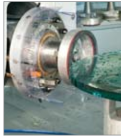
Cup wheel edging Mola a tazza - Meule boisseau Topscheiben - Muela de copa
